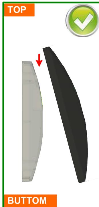
Above picture shows the correct direction (TOP) that outer housing needs to be applied.
