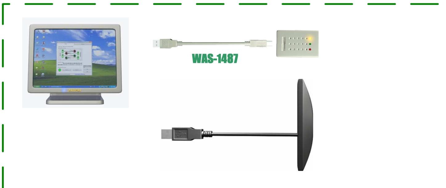
Please have two USB port in your computer. Connect URkit to one USB port as a key to access the software. Connect UR reader to another USB port and run software for configuration. Please don't remove URKit before you finish the configuration with UR reader.
