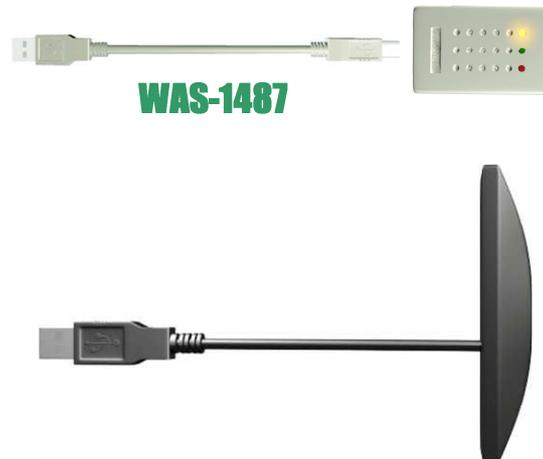
Please have two USB port in your computer. Connect URkit to one USB port as a key to access the software. Connect UR reader to another USB port and run software for configuration. Please don't remove URkit before you finish the configuration with UR reader.
